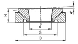
$\begin{array}{lll} D & = 105 \\ d & = 58 \\ d1 & = 78 \\ H & = 25 \\ Max \ screw \ dimension = M48 \\ Static \ load \ (kN) & = 546 \\ Weight \ (g) & = 430 \\ \end{array}$
